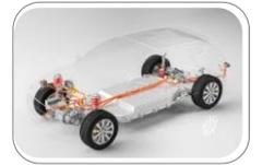
④ Battery Pack (Mounted on electric vehicles)
